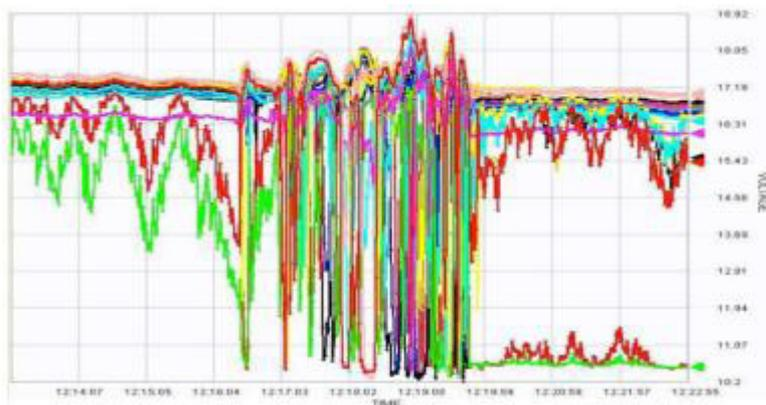
This example shows that even though the direct impact of transient cloud cover might be short in duration, it can cause disproportionate reduction in energy output due to the persistent limitations of the central MPPT algorithm.
